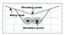
Figure.2: Representation of two front gears that are responsible for moving the links to and fro.
